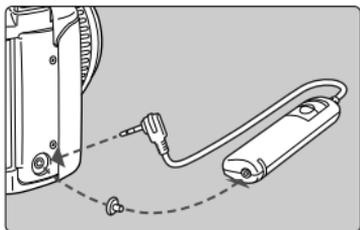
Connect the Remote Switch RS-60E3's (sold separately) plug to the camera's remote control terminal. To take a picture, press the Remote Switch's shutter-release button.
