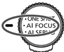
The AI Focus AF mode switches automatically from One-Shot AF to AI Servo AF if the subject starts to move. If focus is achieved in the One-Shot AF mode and the subject starts to move continuously, the camera will detect the movement and switch automatically to AI Servo AF to focus track the subject.
