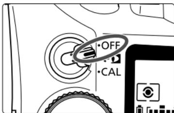
Turn the Eye Control switch to <OFF>. The AF point can then be selected automatically or manually.
