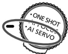
**While you press the shutter button halfway, the camera focuses continuously**
