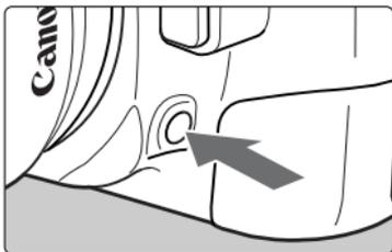
Press the depth-of-field preview button to stop down to the current aperture setting. The diaphragm in the lens will be set to the current aperture so you can check the depth of field (range of acceptable focus) through the viewfinder.
