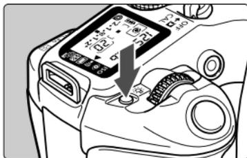
LCD panel illumination is provided. Press the <☀> button to illuminate the LCD panel for about 5 sec. The illumination can be turned off by pressing the button again. Turn on the illumination when it is too dark to see LCD panel. The illumination turns off automatically after the picture is taken.
