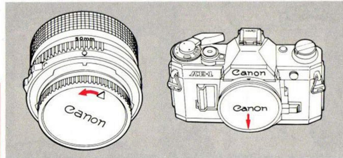
Remove the rear lens cap by turning it in the direction of the arrow until it stops and pulling it out.
