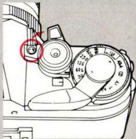
Push the self-timer lever forward to uncover the self-timer lamp.
