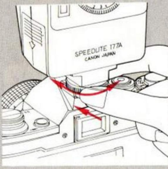
Load the flash with batteries and slide it into the AE-1's accessory shoe. Tighten the lock nut.
