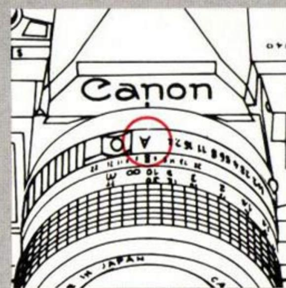
While pressing in the EE lock pin, turn the aperture ring in the direction of the arrow until "A" click-stops at the aperture index. "A" will be in line with the red dot on the camera. If you forget to do this, automatic exposure will be impossible.
