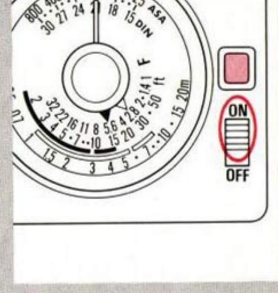
Turn the Speedlite's main switch ON. After the pilot lamp glows, press the shutter button to take the picture.
