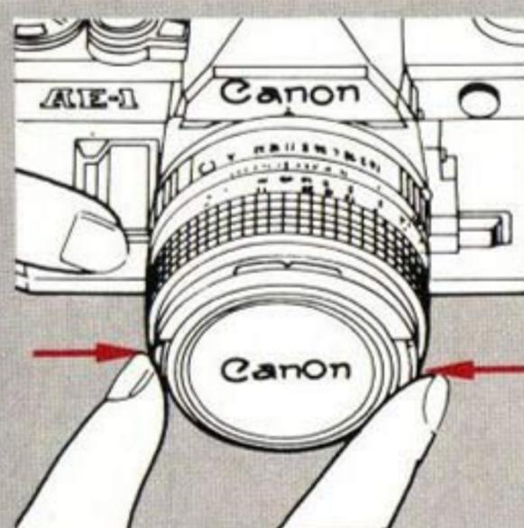
Remove the front lens cap.
