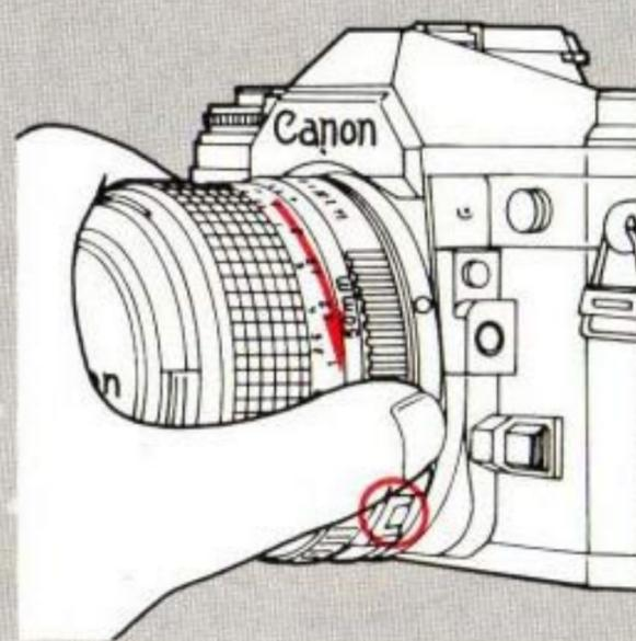
Make sure the lens release button has popped out. Otherwise, the lens will not work properly. DO NOT press the lens release button while mounting or it will not pop out.
