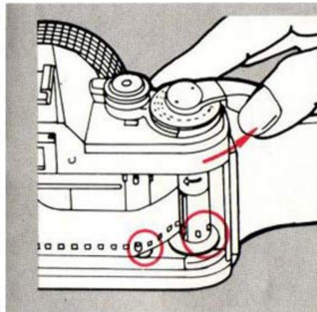
Advance the film once. Check that the film perforations are engaged in the teeth of the film transport sprocket and the take-up spool.
