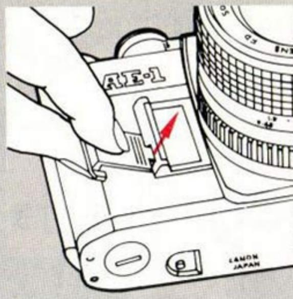
Open the battery chamber cover using the viewfinder cover.
