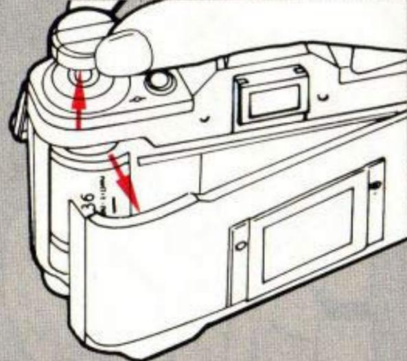
Then open the back cover, remove the film cartridge, place it back in its canister and have it developed as soon as possible.
