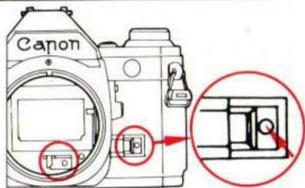
**☑** When film is loaded, make sure it is completely advanced to the next frame before mounting the lens.
