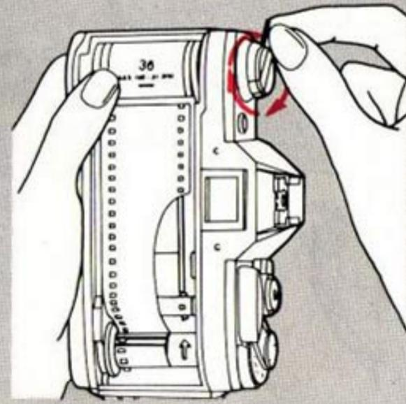
The film should be taut. If there is slack, gently turn the rewind crank in the direction of the arrow until it stops. Close the back cover.
