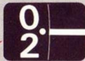
Take several blank shots, releasing the shutter and advancing the film, until the frame counter reads "1" (the dot following zero). While doing this, keep an eye on the rewind knob. If it rotates in the direction of the arrow, the film is loaded correctly.
