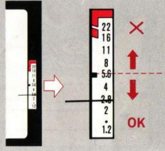
If the battery is good, the meter needle will rest at or below the battery check index. If there is not enough power, it will rest above the index. Replace the battery.
