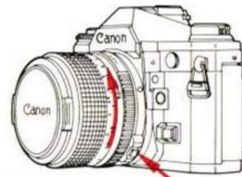
To remove the lens, turn it in the direction of the arrow, while pressing the lens release button, until it stops.
