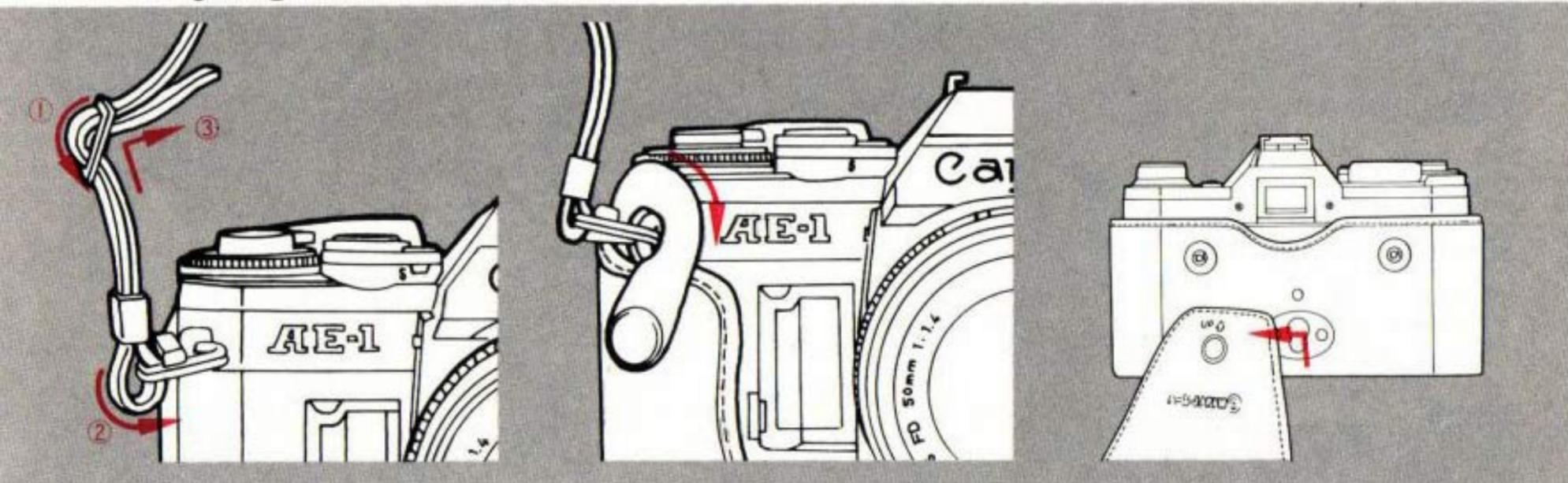
Thread the ends of the strap through the rings on the camera as shown.
