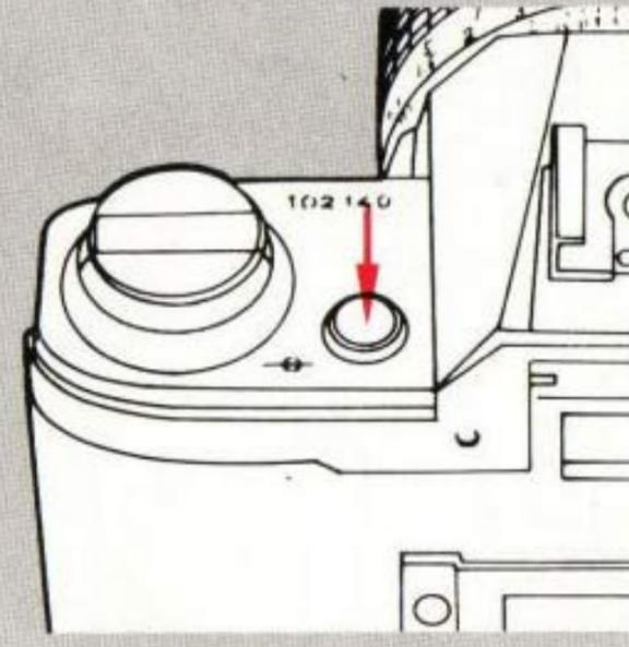
Press the battery check button while looking through the viewfinder. The meter needle in the viewfinder will move.
