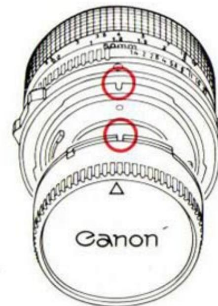
To reattach the rear lens cap, align it with the lens as illustrated. Then lightly push it in and turn it clockwise until it stops.
