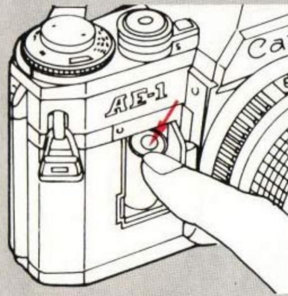
Insert the negative end first. Then push down and insert the positive end. Close the chamber cover.
