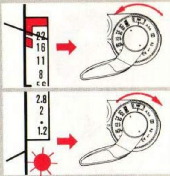
Set a shutter speed by turning the shutter speed dial until a number from 60 to 1000 is aligned with the index.
