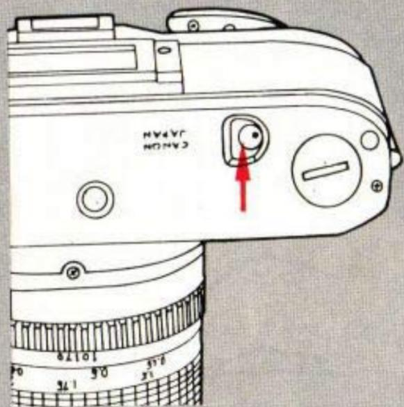
You can tell you have reached the end of the film by the frame counter and the film advance lever. Either the film advance lever will not turn at all or it will not turn all the way. First press in the rewind button. You may immediately let go of it.
