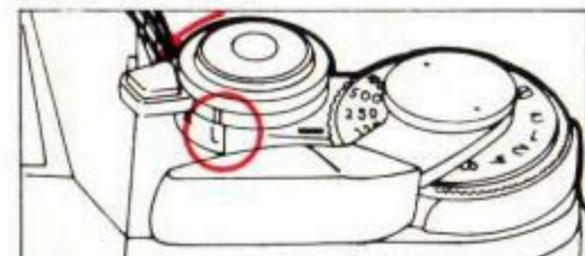
✓ Turn the shutter button lock lever to "L" to prevent accidental shutter release or battery drain whenever you are not using the camera.
