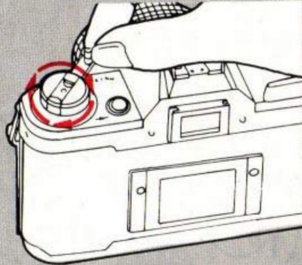
Then turn the rewind crank in the direction of the arrow until the frame counter, which counts backwards as you rewind, reaches "S".
