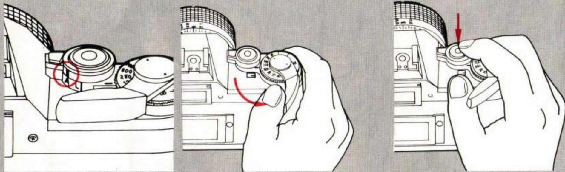
Turn the shutter button lock lever to "A".
