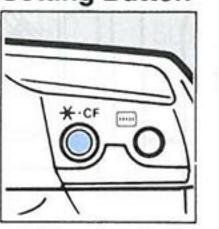
Pressing this button locks in the current exposure reading and allows recomposition without changing the expo-
