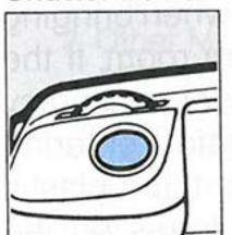
The shutter button has a two step construction. Press halfway (to the first step) to activate focusing and meter-
