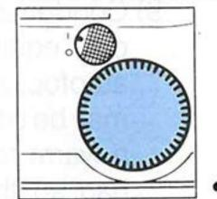
Use for operations such as selecting the aperture value in manual exposure mode and setting exposure com-
