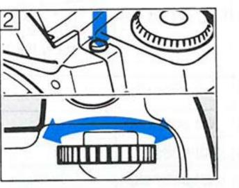
This function lets you vary the automatic flash exposure level of the built-in flash and EOS external flash units. The flash exposure can be compensated up to ±2 stops in 1/2-stop increments.
