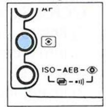
Press this button and operate the main dial to select the desired metering mode Evaluative metering,
