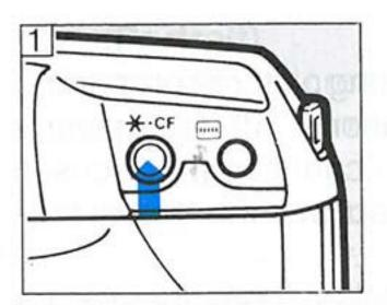
When you press the AE lock button, \*\*lights in the viewfinder to indicate that AE lock is set. Once \*\* appears the exposure remains locked even if you release the AE lock button. AE lock is available in P, Tv, Av and DEP shooting modes.
