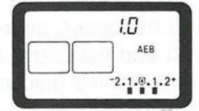
Auto exposure bracketing is particularly effective when using slide film, which produces noticeably different results with even small exposure variations.
