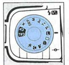
Turn to select the shooting mode. Setting the dial to the "L" position locks the dial and turns off the power. To
