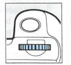
Use in conjunction with other buttons for operations such as selecting the focusing mode, film winding mode,
