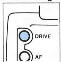
Press this button and operate the main dial to select the desired film winding mode
