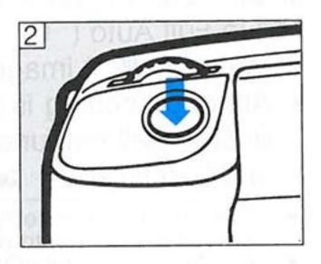
When the red-eye reduction function is set and the shutter button is pressed halfway, the bar indicators in the LCD panel and viewfinder light up for about 1.5 seconds. When these indicators go out, press the shutter button completely to take the picture.
