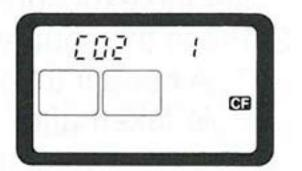
The number in the LCD panel alternates between 0 and 1 each time the custom function set button is pressed.
