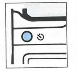
Press to display the " 👏 " symbol in the LCD panel and activate the self-timer. To cancel the selftimer, press
