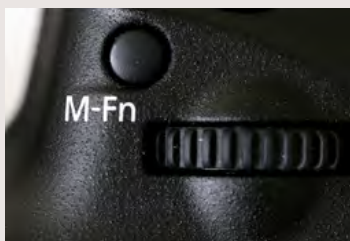
The mode is changed each time the M-Fn button is pressed
