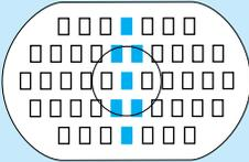
(1) With lenses whose maximum aperture is  $f/2.8$  or faster (lower  $f$ /number), the AF points highlighted in the illustration will be cross-type sensors sensitive to both vertical and horizontal lines. The remaining 38 AF points will only be horizontal-line sensitive. The cross-type sensor's vertical-line sensitivity is three times higher than the horizontal-line sensitivity.
