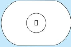
(3) With the following Extenders and L-series lenses whose maximum aperture is faster than f/8, the center AF point will be horizontal-line sensitive only. The other AF points cannot be used for AF.
