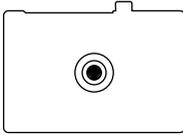
Lenses with a maximum aperture smaller (higher  $f$ /number) than  $f/5.6$  will cause the focusing screen's microprism to darken.
