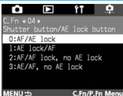
1: You can focus at one location and obtain AE lock at another location in the scene. Press the  $\langle * \rangle$  button to autofocus and press the shutter button halfway to attain AE lock.
