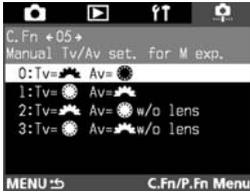
1: This is convenient when you have to often change the aperture during studio sessions with studio flash units. Also, when you use AEB in the manual exposure mode, the shutter speed can stay fixed while only the aperture is shifted for AEB.
