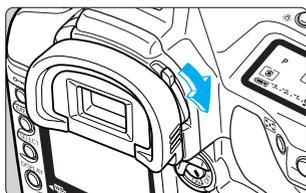
To cover the eyepiece with the eyepiece shutter, turn the lever as shown by the arrow.
