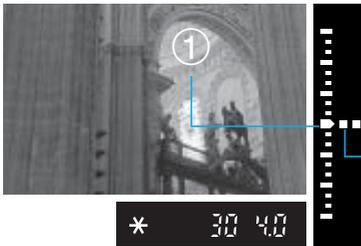
**Exposure level of the first spot meter reading**
