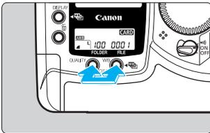
To revert to the camera's default settings, press the **<QUALITY>** button and **<WB>** button simultaneously for 2 sec.
