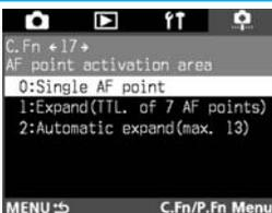
1: The AF point activation area expands by one point all around the manually-selected AF point. A total of 7 AF points become active. This setting is effective for when only one manually-selected AF point is unable to focus track a subject moving erratically.
