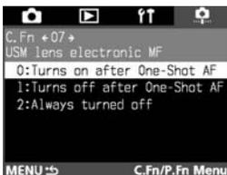
1: This prevents the focus from being thrown off by inadvertent turning of the focusing ring after One-Shot AF. (MF is possible before AF is achieved.) With both C.Fn-07-1 and C.Fn-07-2, manual focusing is possible with the lens focus mode switch set to <MF> (or <M>).
