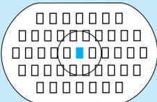
(2) With the following L-series lenses whose maximum aperture is brighter than  $f/4$  by lens only or with Extenders, the center AF point will be a cross-type sensor for high-precision AF. The remaining 44 focusing points will only be horizontal-line sensitive (except with EF 70-200mm  $f/2.8$  USM + Extender EF 1.4x).
