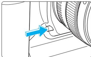
The depth of field is the range of acceptable focus in front of and behind the point of focus. (→p.156) The depth of field changes depending on the aperture. Press the depth-of-field preview button to stop down the aperture and see the range of acceptable focus in the viewfinder.
