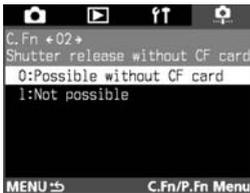
1: With C.Fn-02-1, the shutter button will not work if there is no CF card in the camera. This prevents picture taking without a CF card.
