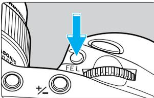
**3** Next, aim the AF point over a highlight area (the window ②) and press the <FEL> button. Do the same for the shadow area (the wall ③).
