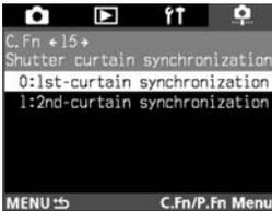
1: By using a slow sync speed, you can create a light trail following a moving subject. The flash fires right before the shutter closes. This Custom Function can be used to obtain 2nd-curtain sync effects even with EX-series Speedlites which do not have this capability. If an EX-series Speedlite having this capability is set for 2nd-curtain sync, it will override this Custom Function.
