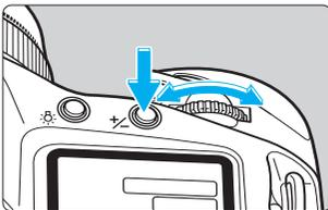
Press the <⚡> button and turn <⚙> dial within (⓪6) to set the desired exposure compensation amount.
