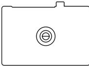
Lenses with a maximum aperture smaller (higher  $f$ /number) than  $f/5.6$  will not cause the focusing screen's microprism to darken.
