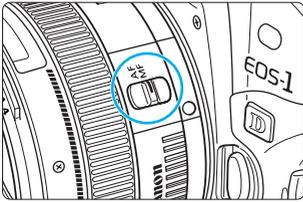
**1** Set the lens focus mode switch to **<MF>** (or **<M>** on older lenses).
