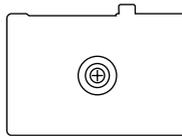
Focus with the vertical and horizontal splits. Lenses with a maximum aperture smaller (higher  $f$ /number) than  $f/5.6$  will cause the focusing screen's split portion to darken.
