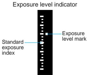
**5** Refer to the exposure level indicator and set the shutter speed and aperture to obtain the desired exposure level.
