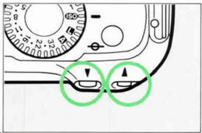
Use this function to check or manually set the film speed. The film speed can be set within a range of ISO 6-6400.
