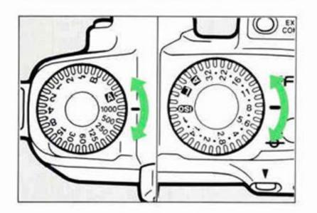
In this mode you set both the shutter speed and the aperture value. Use this mode when using a separate meter or when you wish to purposely vary the exposure.
