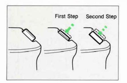
The shutter button has two steps. Pressing the shutter button halfway (to the first step) turns on the viewfinder display. Pressing the shutter button completely takes the picture. Always press the shutter button slowly and gently with the ball of your finger to prevent camera shake.
