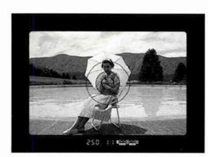
In situations where there is a large difference in brightness between the main subject and background, the subject may not be properly exposed depending on the composition. In such situations use the partial metering button to selectively meter the desired portion of the scene and lock the exposure setting. When partial metering is used the exposure will not change even if the composition is changed.
