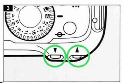
You can compensate the exposure according to the subject conditions when shooting in Program AE, Shutter-priority AE or Aperture-priority AE mode.
