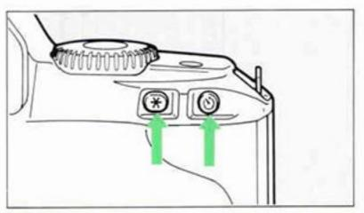
This function lets you rewind and remove the film before the roll is finished.
