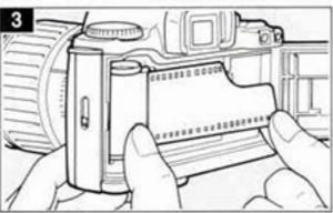
This camera uses a prewind system. When film is loaded, the camera first winds all of the film onto the take-up spool and then rewinds it back into the film cartridge one frame at a time as each picture is taken. The frame counter counts down as pictures are taken, allowing you to always see at a glance how many frames are left. The camera automatically sets the film speed when DX-coded film is loaded.
