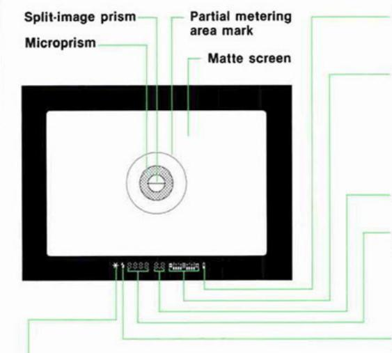
\* (Partial metering/AE lock) indicator
