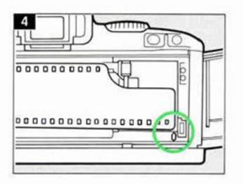
After checking that the film lies flat and that the tip is aligned with the orange mark, close the back cover.
