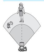
This is fully automatic wireless flash shooting with one external Speedlite and the built-in flash.
