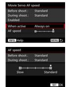
You can set the Movie Servo AF's AF speed and its operation conditions. This function is settable when [Movie Servo AF] is set to [Enable] and [AF method] is set to [FlexiZone - Single]. Additionally, the function is only enabled when using a lens compatible with slow focus transition during movie shooting\*.
