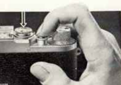
While the shutter is operating the main speed dial revolves. Avoid touching it when pressing the button.
