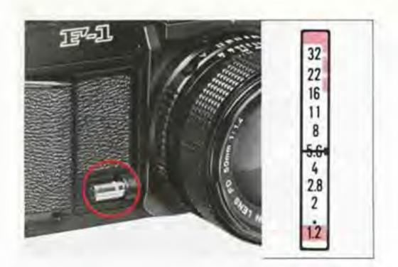
4. Turn the aperture ring (or shutter dial) until the meter needle is aligned with the stopped-down metering/battery check index. Choose a slower speed if the meter needle rests below the index, or a faster speed if the meter needle rests above the index.
