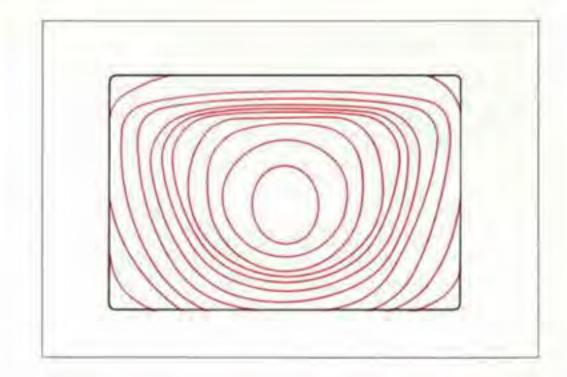
With the New Canon F-1, a special optical element in each focusing screen determines the metering sensitivity area. Thus the metering area can be changed, according to the subject you are shooting and the lens in use, simply by replacing the focusing screen.
