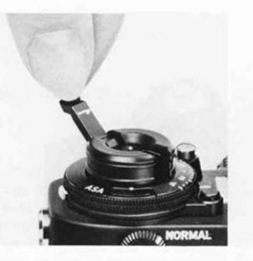
The New F-1's provision for multiple exposures allows you to easily make two or more exposures on the same frame for creative effect.
