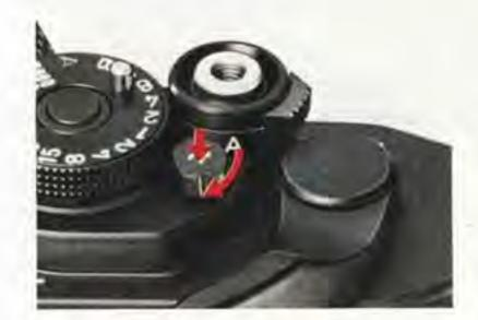
When you have reached the end of the film, the film advance lever will stop before the end of its stroke.
