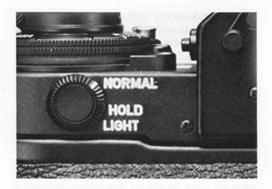
HOLD: The meter turns on the moment you press the shutter button half-way and stays on for 16 seconds even if you remove your finger from the shutter button. It automatically turns off after the specified time, thus conserving battery power. This mode is particularly suited for manual exposure and any situation in which you need
