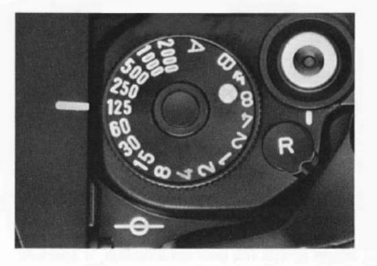
The New Canon F-1's hybrid shutter is electronically as well as mechanically controlled. Shutter speeds from 1/2000 to 1/125 sec., "\$" (1/90 sec.) and "B" (bulb) are mechanically governed, while 1/60 to 8 secs. are electronically controlled. With the AE Finder FN attached and the shutter dial on "A," shutter speeds from 1/1000 to 8 secs. are electronically controlled.
