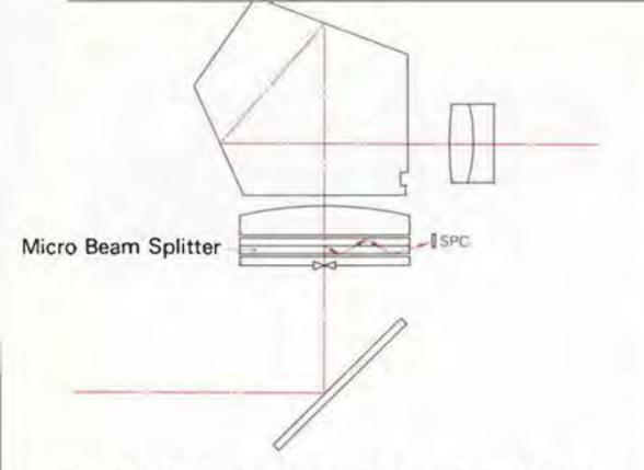
Since the optical element is located in close proximity to the focal plane, this new system of metering sensitivity distribution ensures extremely accurate results.
