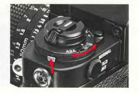
Turn the setting dial, while pressing the lock release button, until the desired film speed aligns with the index. The dial cannot be turned lower than ASA 6 or higher than ASA 6400. The table on the next page shows the ASA/ISO film speeds which can be set on the New Canon F-1. Figures in parentheses are intermediate speeds which are indicated by dots on the ASA/ISO dial.
