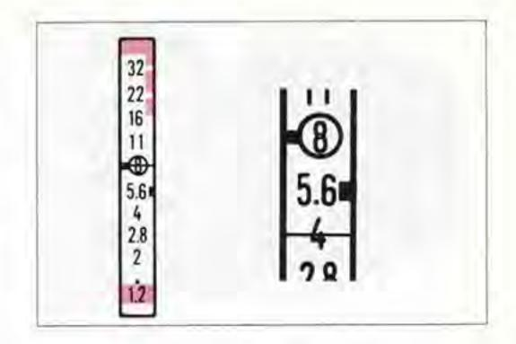
equivalent to one f/stop. This method of exposure correction is useful, for example, when shooting a subject with strong backlight.
