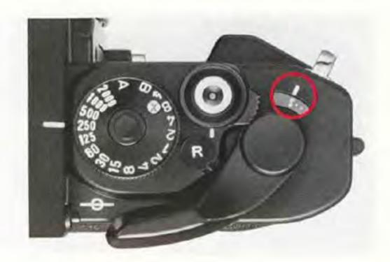
Each time you advance the film, the frame counter also advances to the next number. It can count up to 39 frames. The numbers 1, 12, 20, 24 and 36 are in orange, the latter four to call your attention to the fact that rolls with those numbers are or are almost finished. The frame counter automatically returns to "S" when you open the camera back. During multiple exposures, the frame counter advances each time you wind the advance lever.
