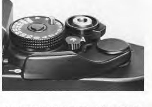
The battery check button also serves to cancel the self-timer, meter reading, illumination of viewfinder information ("LIGHT" setting of meter mode selector), and shutter operation during long exposures. The circuit is cancelled the moment you press the button, and the second curtain will close when you remove your finger. The shutter will not be released if you press the shutter button while pressing the battery check button.
