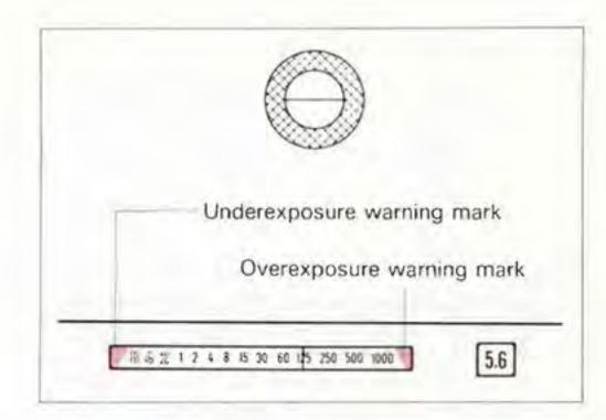
There is a possibility of camera movement if the meter needle indicates a shutter speed of 1/30 sec. or slower. In this case, choose a larger aperture until the shutter speed indicated is 1/60 sec. or faster. If you have set the maximum aperture and the shutter speed is still slower than 1/60 sec., attach the camera to a tripod, use a flash or add artificial light.
