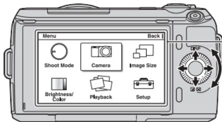
When options are displayed on the screen, you can browse through them by turning or pressing the top/bottom/left/right parts of the control wheel. Press the center to make your choice.
