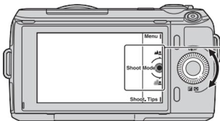
The arrow means you can turn the control wheel.
