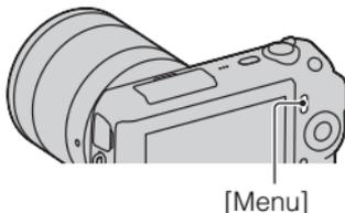
2 Use the control wheel to select [Shoot Mode] → desired mode, and press the center.
