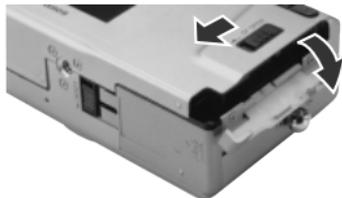
2. As shown below, orient the card with its label side facing up and insert it into the slot until it is firmly seated.
