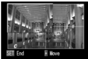
After the indicator stops flashing green, the fourth recorded image will display in the upper left, and a preview of a new photographic subject captured by the lens will appear in the position of the first image.
