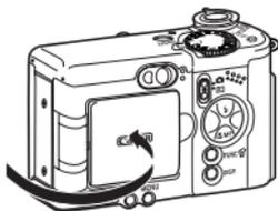
The LCD monitor will automatically turn off when it clicks shut against the camera body. For protection, always close the LCD monitor after use.
