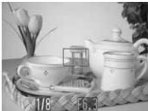
The correct exposure has been set if the shutter speed and aperture value show in white.
