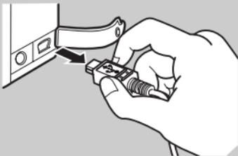
To disconnect the cable from the camera: Hold the cable connector firmly at both sides and pull it straight out.
