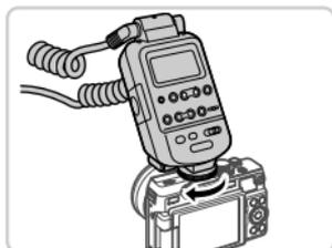
**3 Attach the controller to the camera.**
