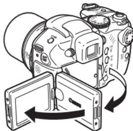
2. LCD monitor is opened to the left 180 degrees and tilted 180 degrees toward the lens.
