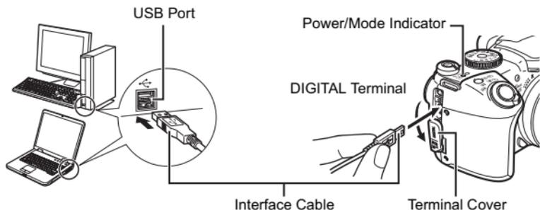
When the power is turned on automatically, the camera and computer will be able to communicate. (The LCD monitor or viewfinder turns off, and the power/mode indicator lights yellow.)
