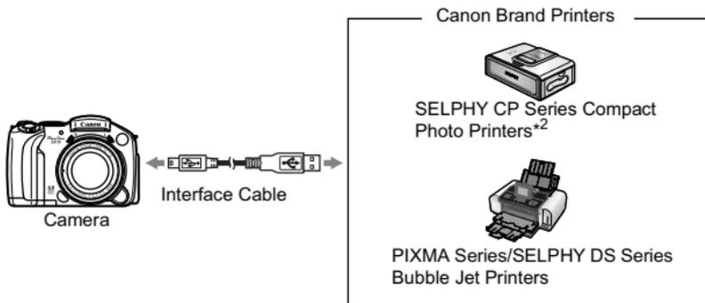
\*1 Since this camera uses a standard protocol (PictBridge), you can use it with other PictBridge-compliant printers in addition to Canon-brand printers.
