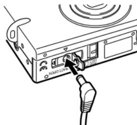
**3** Open the DC coupler terminal cover and attach the cord to the DC terminal.
