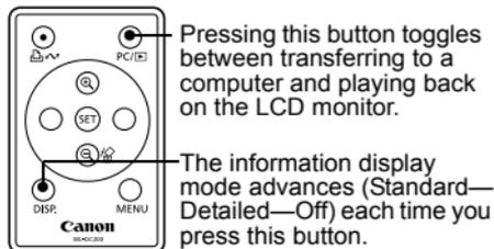
Other than the operations listed above, all of the buttons perform the same functions as the corresponding buttons on the camera.
