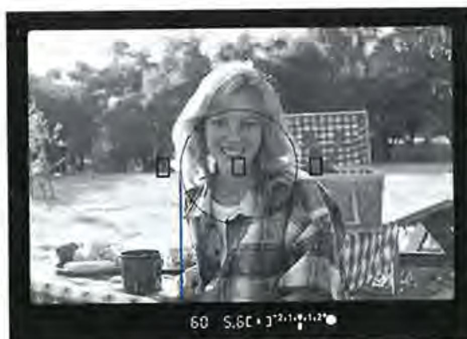
Partial metering circle
