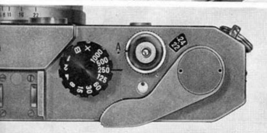
One stroke motion of lever on top of the camera winds the film, cocks the shutter, and advances Exposure Counting Dial. Now the shutter is ready to be released. The shutter release button cannot be released accidentally unless the shutter is completely cocked.
