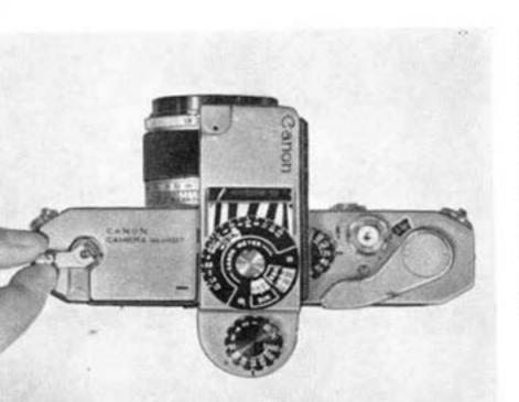
3. Unloading film with the meter mounted on the camera can be done by turning the meter a half-circle clockwise as shown on the left. The meter can be shifted after pulling out the combination dial.
