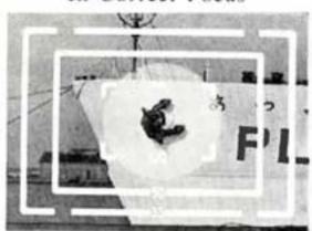
upon should coincide. At this point of coincidence your camera is in focus for the object you are about to photograph.
