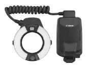
• Macro Ring Lite MR-14EX EOS-dedicated macro ring flash featuring twin flash tubes, Guide No. 14 (at ISO 100 in meters), and E-TTL autoflash. You can fire only one or both flash tubes and control the flash ratio to easily obtain sophisticated lighting effects with E-TTL autoflash. Also, highspeed sync (FP flash), FE lock, and a wireless, multi-Speedlite (with 550EX as a slave) system are possible to
