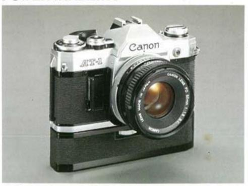
To keep pace with fast action, a great Canon accessory, the Power Winder A, will automatically advance the film at a rate of approximately two frames per second. To continuously advance the film, merely press the shutter release button. A succession of shots may then be taken under constant exposure conditions. Use of the Power Winder A minimizes film winding time and camera movement and gives maximum utilization of all the AT-1's fantastic features.
