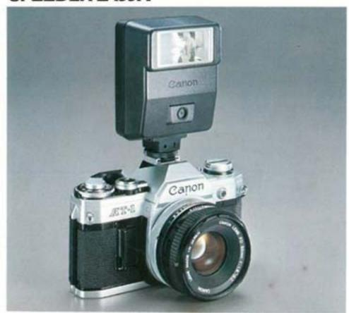
The Speedlite 155A is an electronic flash which can be used for either the Canon AE-1 or AT-1 cameras. Once mounted, with the prescribed aperture set manually, the shutter's synchronization is automatically set at 1/60 of a second except when the shutter speed dial is set at "B". An electronic light sensor located on the front of the 155A automatically controls flash duration. A neon lamp lights when the Speedlite 155A is fully charged and ready to take perfect flash photographs.
