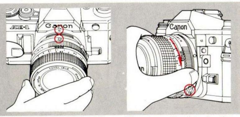
Make sure the lens release button has popped out. Otherwise, the lens will not work properly. DO NOT press the lens release button while mounting or it will not pop out.
