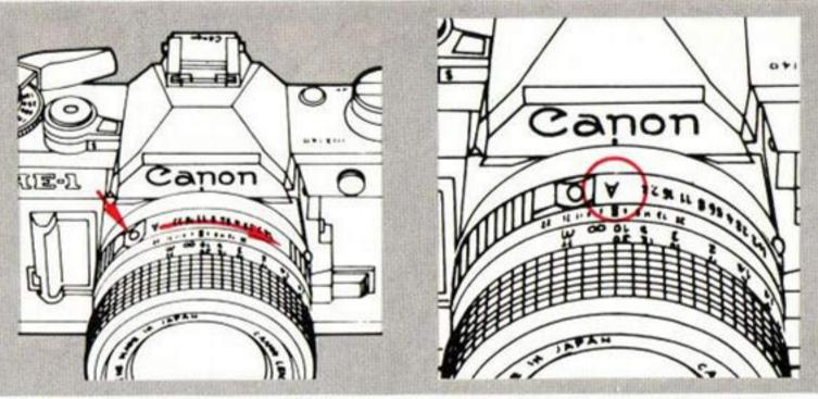
While pressing in the EE lock pin, turn the aperture ring in the direction of the arrow until "A" click-stops at the aperture index. "A" will be in line with the red dot on the camera. If you forget to do this, automatic exposure will be impossible.
