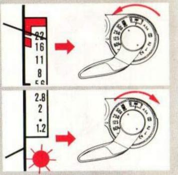
Then look into the viewfinder and press the shutter button HALFWAY. The meter needle will move to tell you whether the shutter speed you have set will give correct exposure. If the meter needle points to the red zone at the top of the scale or if the red LED (Light-Emitting Diode) blinks below the scale, turn the shutter speed dial as shown. Otherwise, exposure will be correct at the shutter speed you have set.
