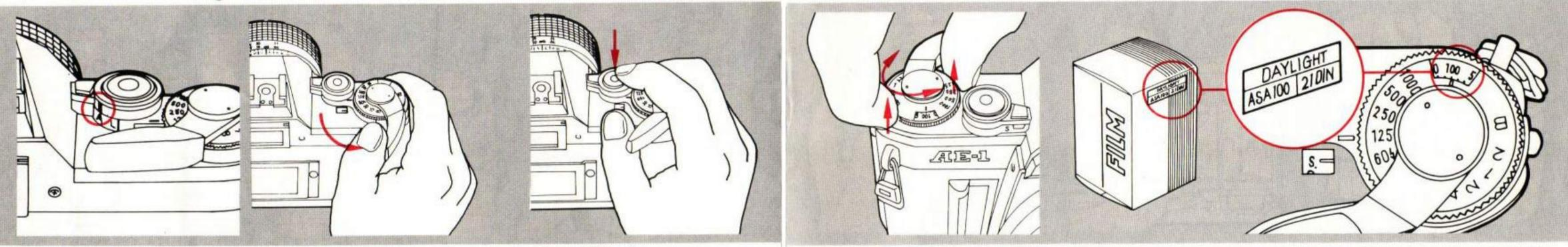
Turn the shutter button lock lever to "A".
