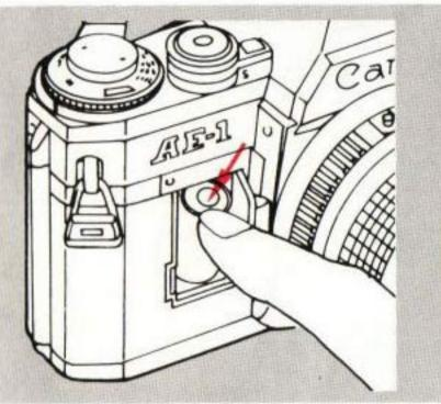
Insert the negative end first. Then push down and insert the positive end. Close the chamber cover. Press the battery check button while looking through the viewfinder. The meter needle in the viewfinder will move. If the battery is good, the meter needle will rest at or below the battery check index. If there is not enough power, it will rest above the index. Replace the battery.
