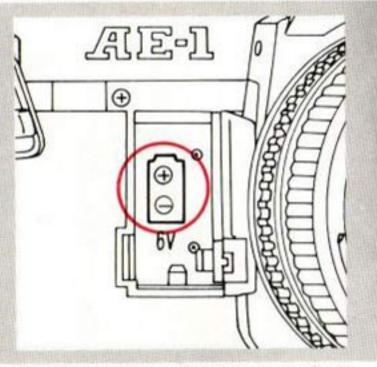
Load one new battery so that its poles are in the directions indicated by the diagram inside the battery chamber.
