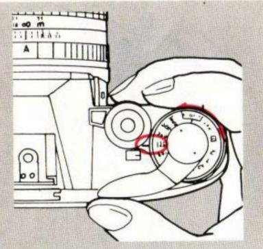
Set a shutter speed by turning the shutter speed dial until a number from 60 to 1000 is aligned with the index.
