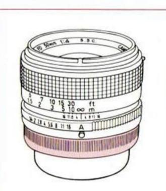
The instructions in this section concerning the lens are for an FD lens without a chrome mount If your lens looks like this with a chrome mount ring, read its instructions for handling the rear cap and mounting it on the camera.
