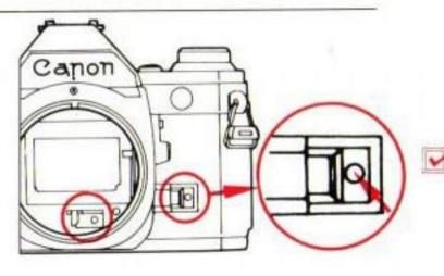
When film is loaded, make sure it is completely advanced to the next frame before mounting the lens.
