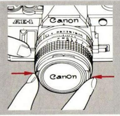
Remove the front lens cap.
