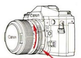
To remove the lens, turn it in the direction of the arrow, while pressing the lens release button, until it stops.
