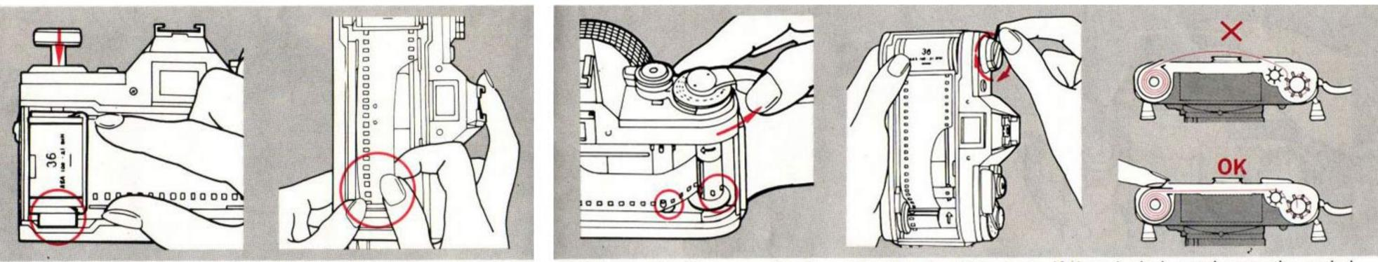
The AE-1 uses color (negative or slide) or black and white film in standard 35mm cartridges. Place the cartridge in the film chamber as shown. Then push the rewind knob down, rotating it until it drops into its normal position. Pull the film leader across the camera and insert it into any slot of the take-up spool.
