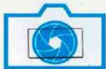
The shutter clicks. The diaphragm closes down to preset f/stop.
