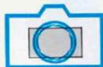
The diaphragm returns to maximum opening.
