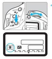
While pressing the < 35 button, turn the <  $\triangle$  > dial until the desired metering mode icon appears.
