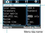
Hold down < SELECT> and turn the < > dial to select a setting. When the desired menu setting is selected, let go of the < SELECT> button. The setting will then take effect immediately. To exit the menu, press the <MENU> button.
