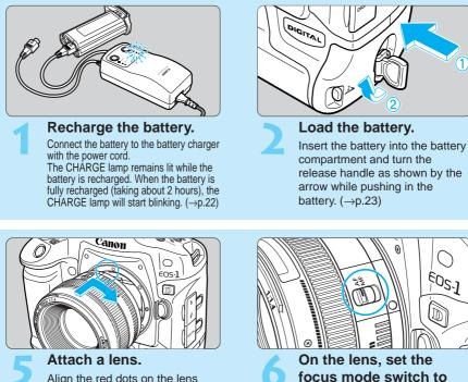
Align the red dots on the lens and camera and turn the lens as shown by the arrow until it snaps in place. ( $\rightarrow$ p.26)
