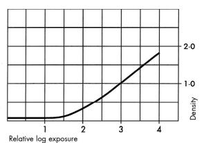
100 DELTA Professional rollfilm developed in ILFORD ID-11 stock for 8<sup>1/</sup><sub>2</sub> minutes at 20°C/68°F with intermittent agitation. This curve is also representative of the 35mm and sheet film formats.
