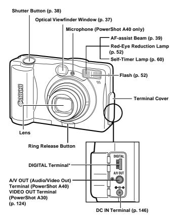
\* If connecting to your computer, use the dedicated USB cable included with the camera (pp. 104, 128). If connecting to a printer, use the direct interface cable DIF-100 included with the printer. (For a list of printers that work with this camera, please refer to the System Map.)
