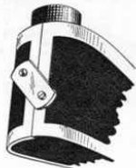
Illustration 2 Turn latch as shown as far as it will go. Do not force.
