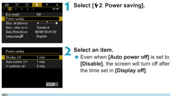
[Display off] and [Auto power off] settings do not apply when Eco mode is set to [On].
