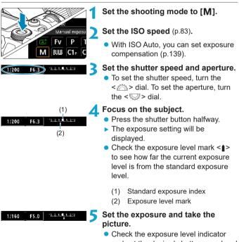
Check the exposure level indicator and set the desired shutter speed and aperture.
