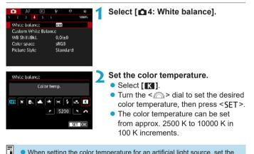
• When setting the color temperature for an artificial light source, set the white balance correction (magenta or green bias) as necessary.
