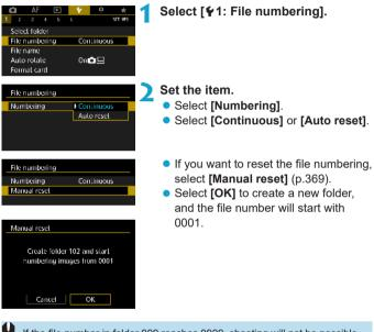
If the file number in folder 999 reaches 9999, shooting will not be possible even if the card still has storage capacity. The screen will display a message telling you to replace the card. Replace it with a new card.
