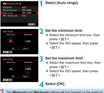
The **[Minimum]** and **[Maximum]** settings will also function as the minimum and maximum speeds for ISO speed safety shift (p.545).
