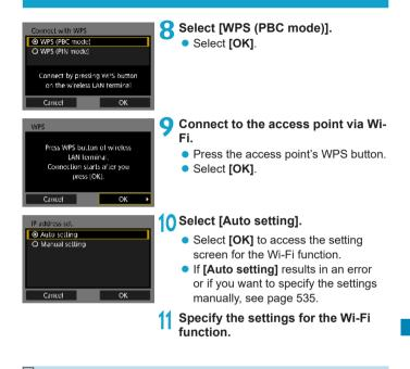
The IP address can only be set automatically in environments using DHCP servers, or access points or routers with DHCP server functionality, and IP addresses, etc. are set to be assigned automatically.
