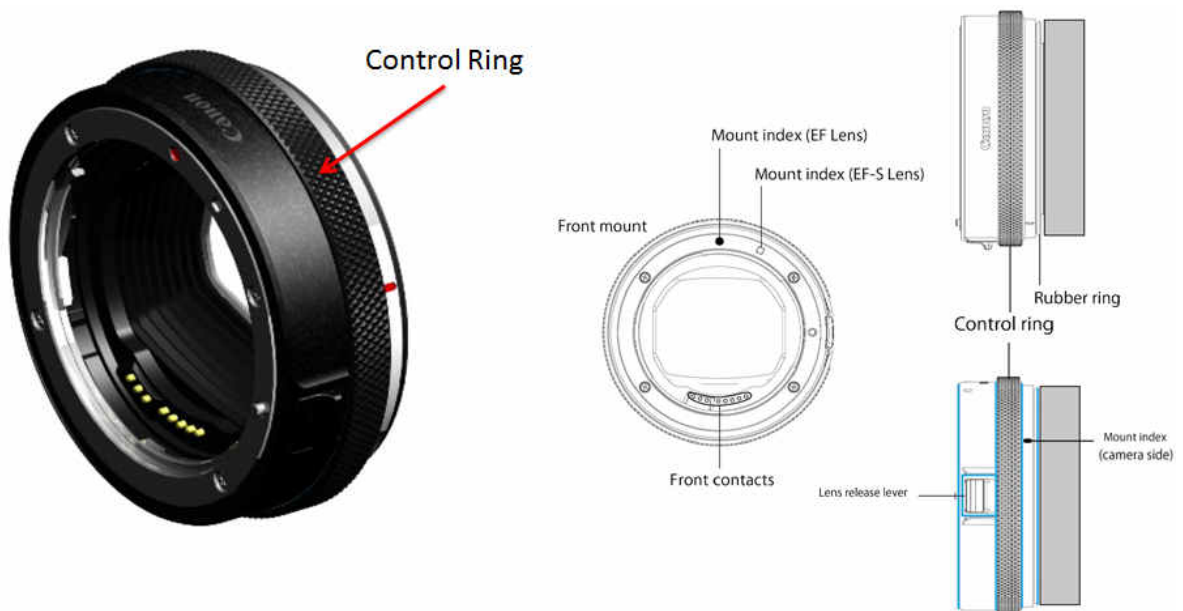
Figure 36 Control Ring Mount Adapter EF-EOS R that incorporates the control ring
