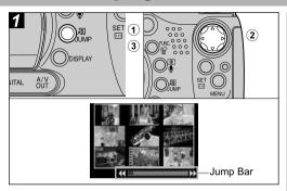
①Press the JUMP button while in single image playback (p. 39) or index playback (p. 41).
