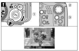
①Turn the mode lever to the right to set the camera to Playback mode.
