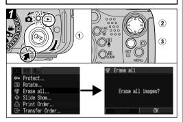
1) Turn the mode lever to the right to set the camera to Playback mode.
