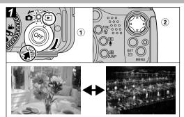
Turn the mode lever to the right to set the camera to Playback mode.
