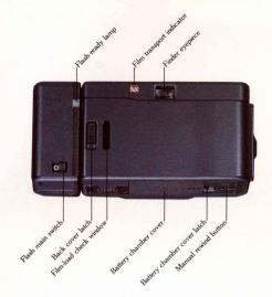
Film Speed Scale: ISO 64, 100, 200, 400, and 1000. Power Source: Two AAA-size alkaline(LR03) or carbon-zinc batteries. Ni-Cd batteries cannot be used. Battery Life: Approx. 30 rolls of 24-exposure film. (Assumes use of new alkaline batteries at normal temperature.)
