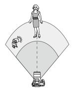
Fully automatic wireless flash photography using one receiver and one sender. Steps 1-4 and 6 apply to all wireless flash photography.
