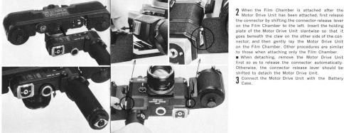
9 When the Film Chamber is attached after the Motor Drive Unit has been attached, first release the connector by shifting the connector release lever on the Film Chamber to the left. Insert the holding plate of the Motor Drive Unit slantwise so that it goes beneath the claw on the other side of the connector, and then gently lay the Motor Drive Unit on the Film Chamber. Other procedures are similar to those when attaching only the Film Chamber.
