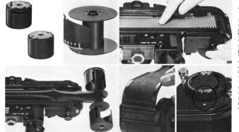
7 Put this take-up magazine into the take-up magazine chamber, in the same manner as the supply magazine was inserted, and push in the magazine attachment knob.
