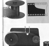
2 Wind a strip film to a spool of the magazine by using Film Loader 250 in a darkroom. Insert a strip film either directly into the supplyside shaft of the Film Loader or by using the spool attached to the Film Loader.
