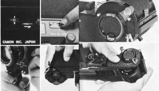
gear. The frame counter counts the number of unexposed frames. Be sure to set the frame counter correctly because it will stop only when the end of the film passes over the film guide roller and will not stop when the counter itself reaches "O". ■ The Motor Drive Unit will not function unless the
