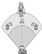
Convenient when you need a large flash output. All the slave units will fire at the same output and be controlled to obtain a standard exposure.
