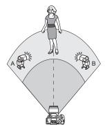
You can divide the slave units into groups A and B, and change the flash ratio to obtain the desired lighting effect. Refer to the Speedlite's instruction manual and set one slave unit to firing group A and the other to firing group B. Position the Speedlites as shown in the illustration.
