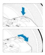
Press a button such as < MODE > or < M-F $\eta$  >, then turn the <  $\stackrel{\sim}{\text{---}}$  > dial. If you press the shutter button halfway, the camera will go back to shooting standby.
