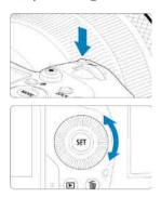
Press a button such as  $< MODE > or < M-F_{\eta} >$ , then turn the  $< \bigcirc >$  dial.
