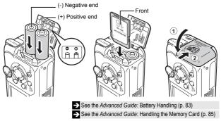
Ensure that the memory card is correctly oriented before inserting it in the camera. It may damage the camera if inserted incorrectly.
