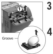
Remove the battery from the holder by pulling it in the direction of the arrow.
