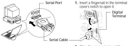
2. Align the arrows to insert the cable into the camera.
