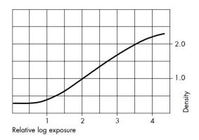
DELTA 400 Professional film developed in ILFORD ID-11 stock for 8 minutes at  $24^{\circ}\text{C}/75^{\circ}\text{F}$  with intermittent agitation.
