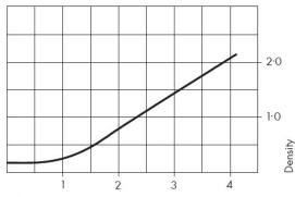
HP5 Plus film developed in ILFORD ILFOTEC HC (1+31) stock for  $6\frac{1}{2}$  minutes at  $20^{\circ}C/68^{\circ}F$  with intermittent agitation. This curve is also representative of roll film and sheet film formats.
