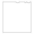
HP5 Plus sheet film is coated on 0.180mm/7-mil polyester base with an anti-halation backing which clears during development. It is available in a wide range of standard sizes. The emulsion faces the user when sheet film is held in the position shown.
