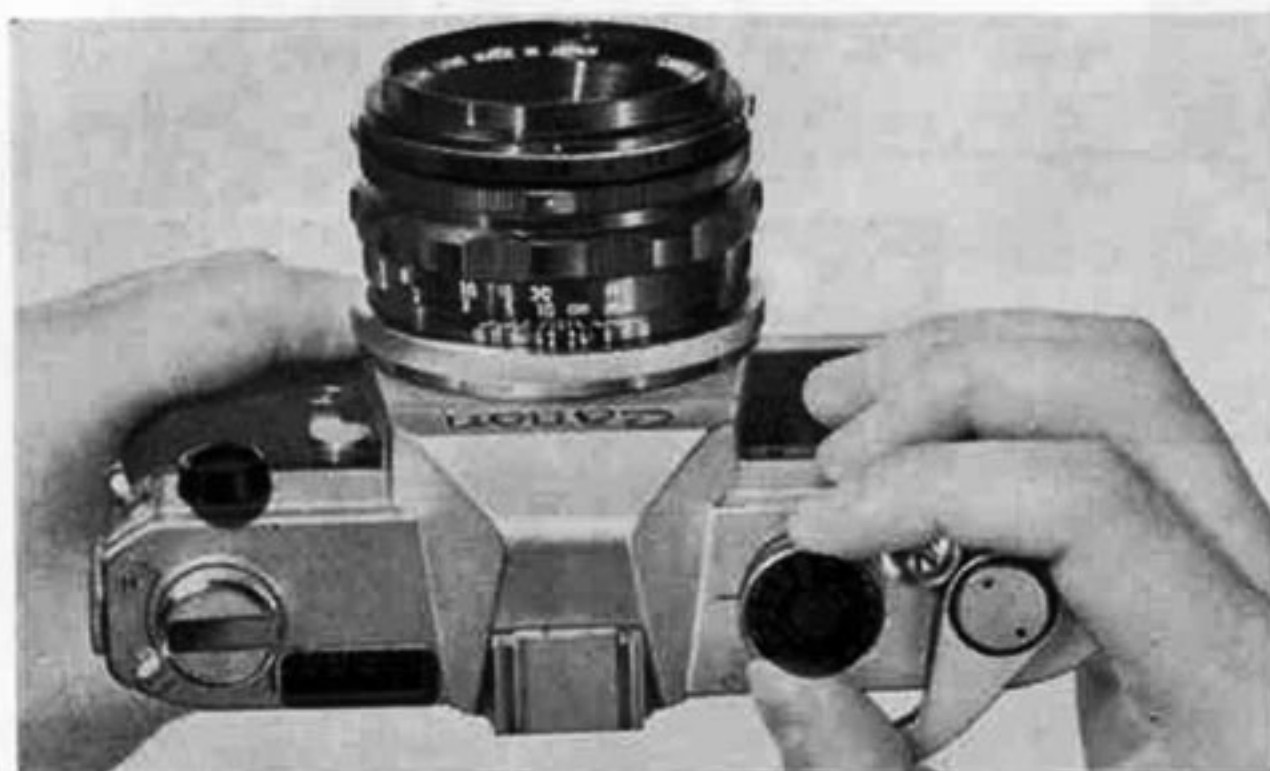
5. Determine the exposure with built-in meter.
