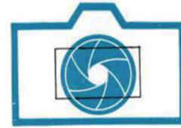
The shutter clicks. The diaphragm closes down to pre-set f/stop.
