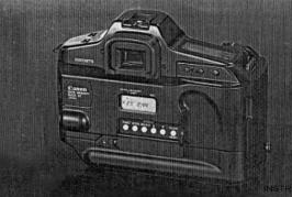
The Data Memory Back 90 is an interchangeable camera back designed for exclusive use with the Canon T90. Simple operations allow you not only to imprint certain types of data automatically on the film, but also to store the various data of your picture and, more, you can check the data after shooting, on the LCD panel.
